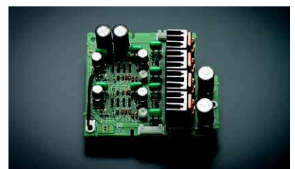
Fully discrete headphone amplifier
