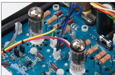
The high voltage triode tube 6FQ7/6CG7 is installed on the output stage.
