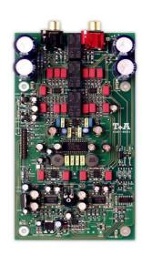
The E-series players are equipped with a D/A converter which is a completely new development; it is of symmetrical construction, with total separation of the two channels. The outstanding feature of our players is their ultra-refined analogue output stages. These offer sound of great beauty, and play a crucial role in the excellent overall quality of reproduction. They process the converted digital sources as well as the analogue sources in the MUSIC PLAYER.
