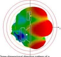
Three-dimensional direction pattern of a conventional loudspeaker, frequency: 2765.0 (Hz)
