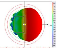
Three-dimensional direction pattern of a loudspeaker with coaxial ELAC X JET, frequency: 2765.0 (Hz)
